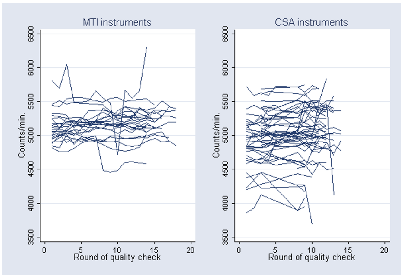
Figure 2 Raw instrument output by round of quality check. Within MTI units variation: SD = 112 counts*min -1 . Between MTI units variation: SD = 195 counts*min -1 . Within CSA units variation: SD = 120 counts*min -1 . Between CSA units variation: SD = 343 counts*min -1 .
