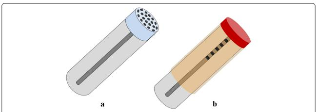
Fig. 3 Schematic representation of the two different types of sensors: with integration and patterning on the tip of the fibre, LOF (a), and based on the long-wheelbase patterns coated with nanoscale layers of functional polymer materials, LPG (b)
