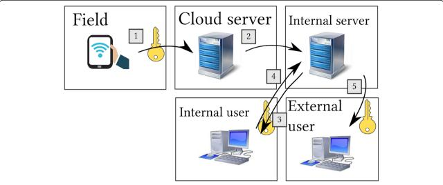
Fig. 2 Data flows: (1) Validated field data are encrypted, submitted to the cloud server, and deleted from the tablet device. (2) Encrypted data are sent via SFTP to an internal storage server. (3) Data are downloaded, decrypted, for checking. (4) Processed data are re-encrypted and re-uploaded. (5) Authorised external users can download and decrypt the data. Key symbol represents encryption/decryption
