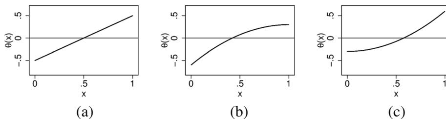
**Fig. 1** Three shapes for  $\theta(x)$  with  $\beta = 1$ . **a**  $\theta(x) = \beta(x - 0.5)$  **b**  $\theta(x) = \beta(0.3 - 0.9(x - 1)^2)$  **c**  $\theta(x) = \beta(-0.3 + 0.9x^2)$
